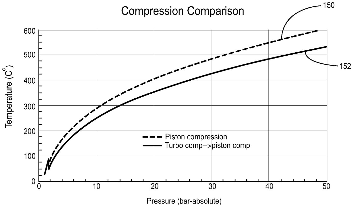
■ For same final compression pressure, after cooling part-way through event reduces final temperature significantly
